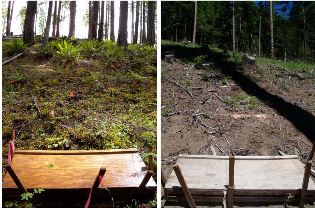
Figure 5.3. Shows contrast between control trap locations (left) and a more heavily disturbed site within the thinned section of the project area (right). Box# 8 is shown on the left and Box #3 is on the right. Note larger amounts of exposed bare soil in Box #3 compared to the control Box #8.
