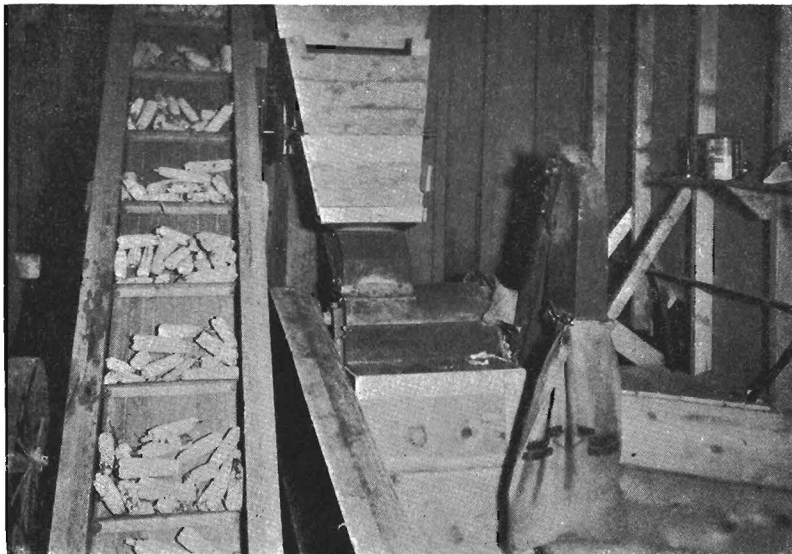
Figure 2. Elevating corn into an ear-corn drier. Cylinder type corn sheller shown at right.
