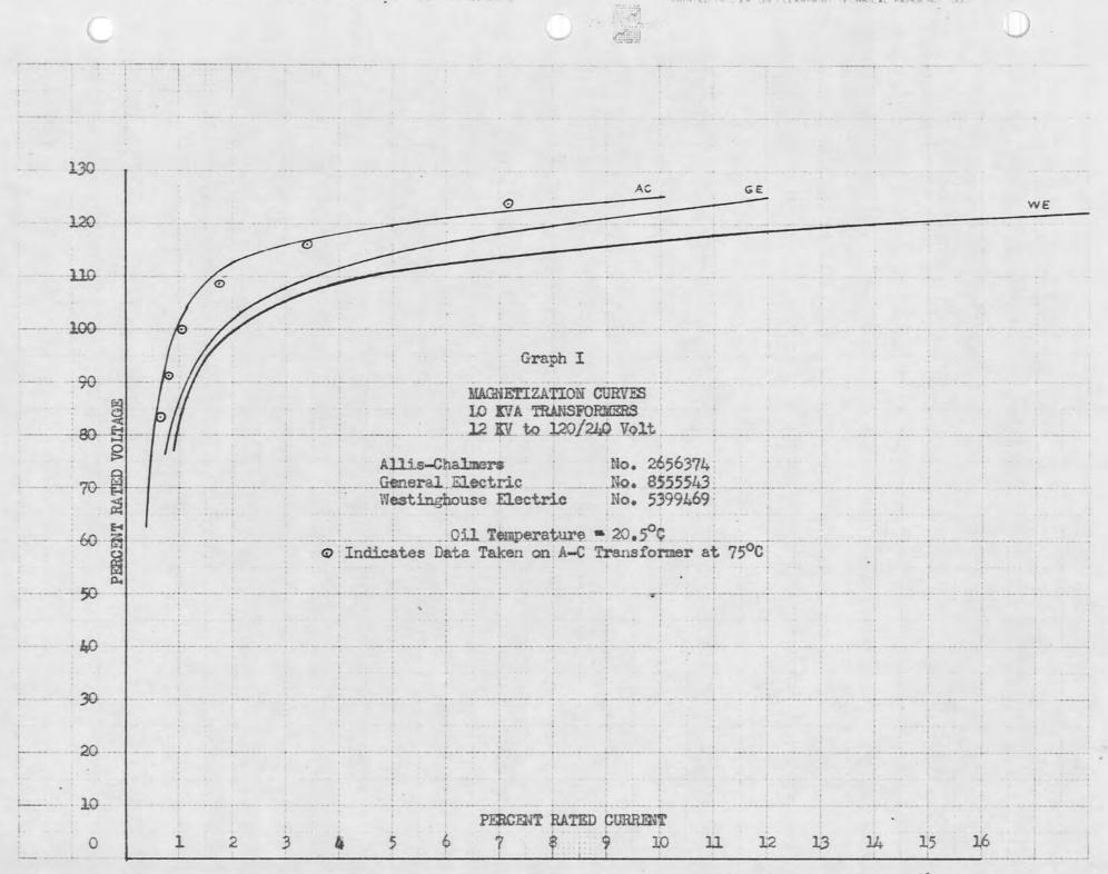
From Graph I, Table 1 was prepared showing the percentage increase in rms exciting current with 116.7% voltage applied. Later in this
