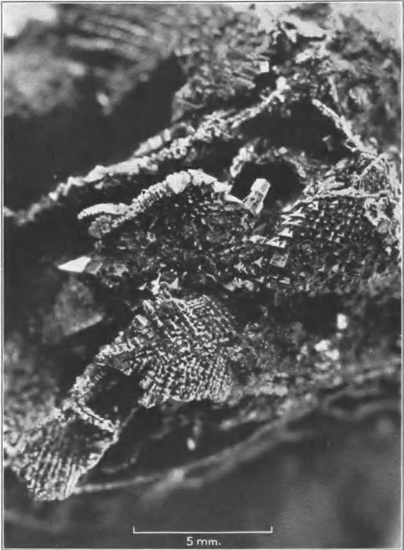
DENDRITIC GOLD FROM LEACHED PART OF VEIN AT BUZZARD MINE, JACKSON COUNTY.
