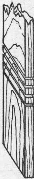
Method of cutting test sections from plank
