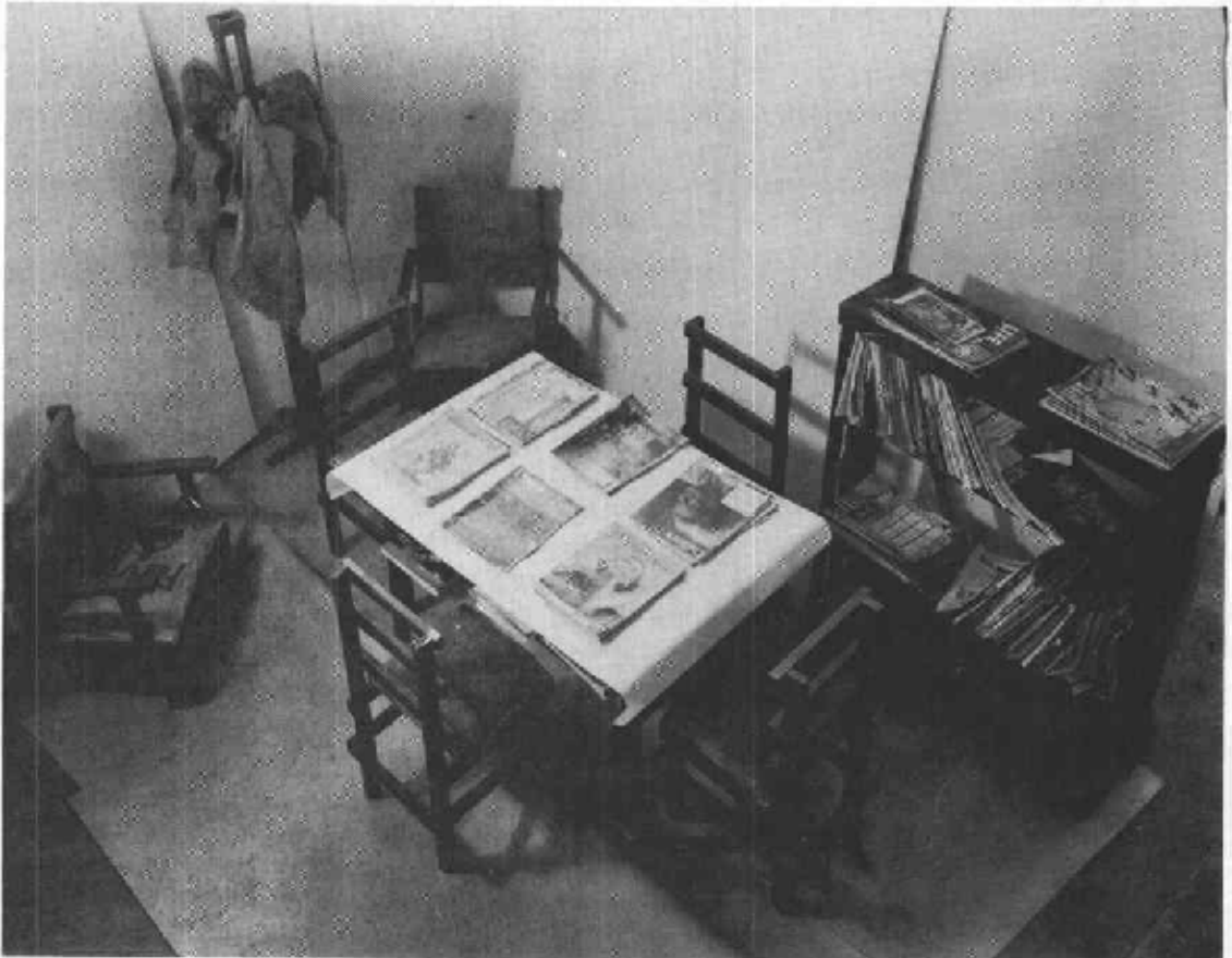
Figure 26. --Dwelling room burn-out test. Interior view showing mock-up furniture used.
