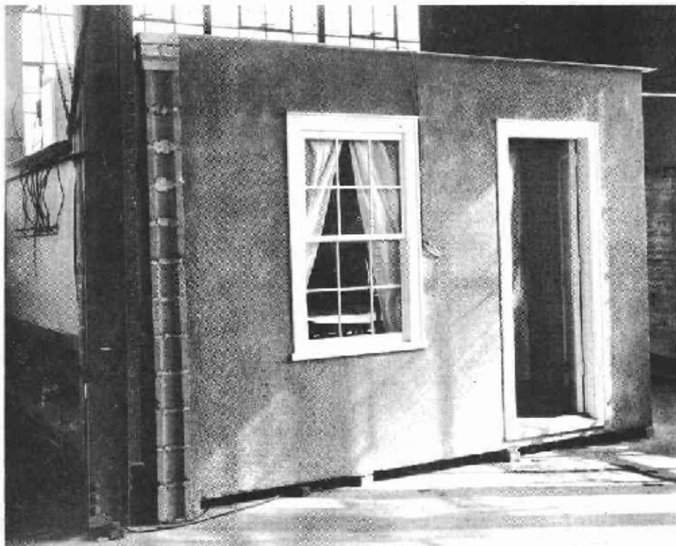
Figure 25. --Dwelling room burn-out test. Exterior view, of room prior to test.
