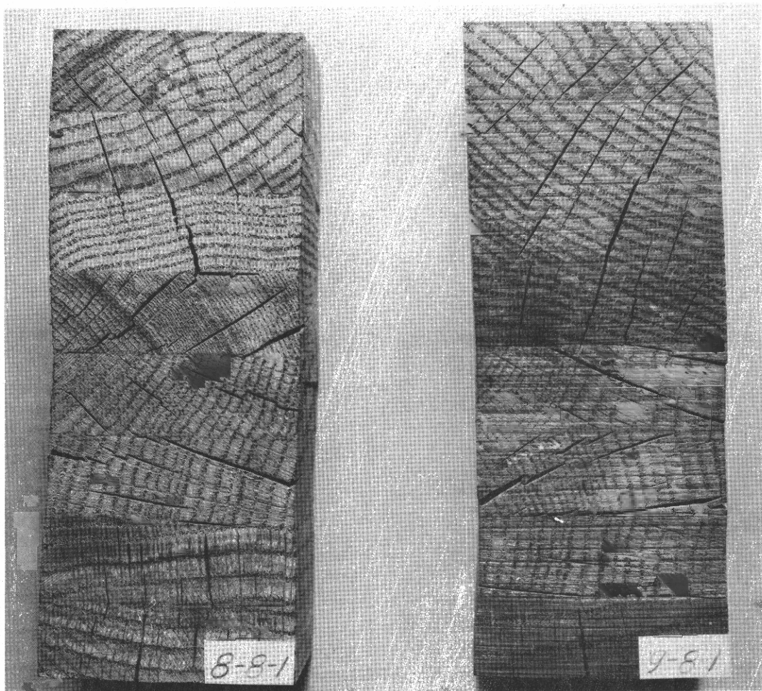
Figure 11.—Sections of laminated red oak beams glued with resorcinol resins cured under pressure for 16 hours at 80° F. (procedure IV) and subjected to three cycles of accelerated soaking and drying. Section on left made with glue H, the one on right with glue I. The wood has checked considerably, but the glue joints are practically free from delamination.
