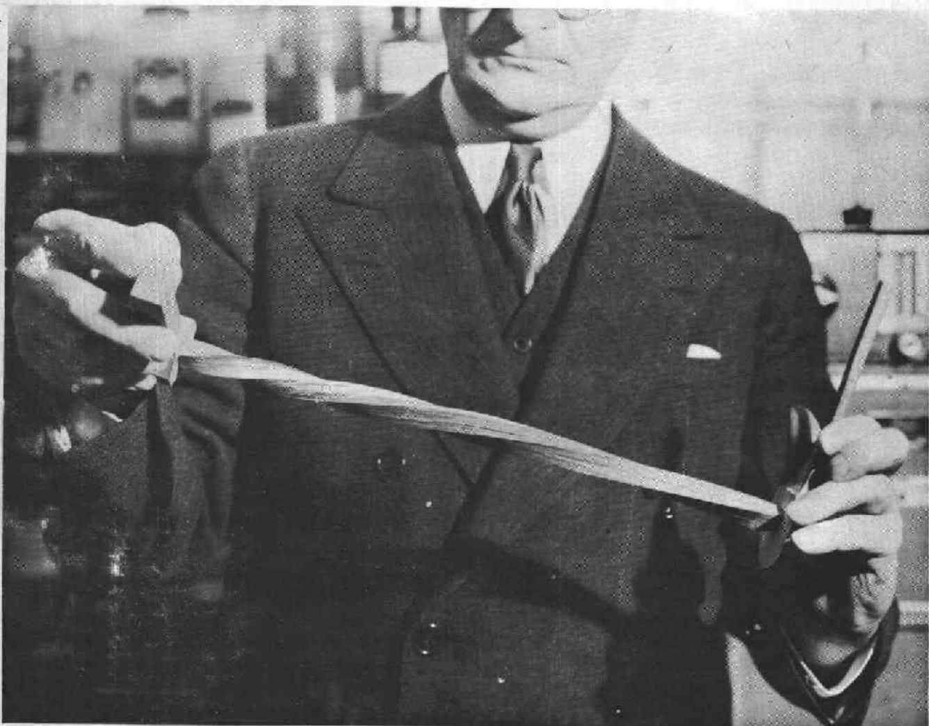
Figure 4.--Urea-treated oak square twisted when hot and retaining twisted shape in which held while cooling and stiffening.
