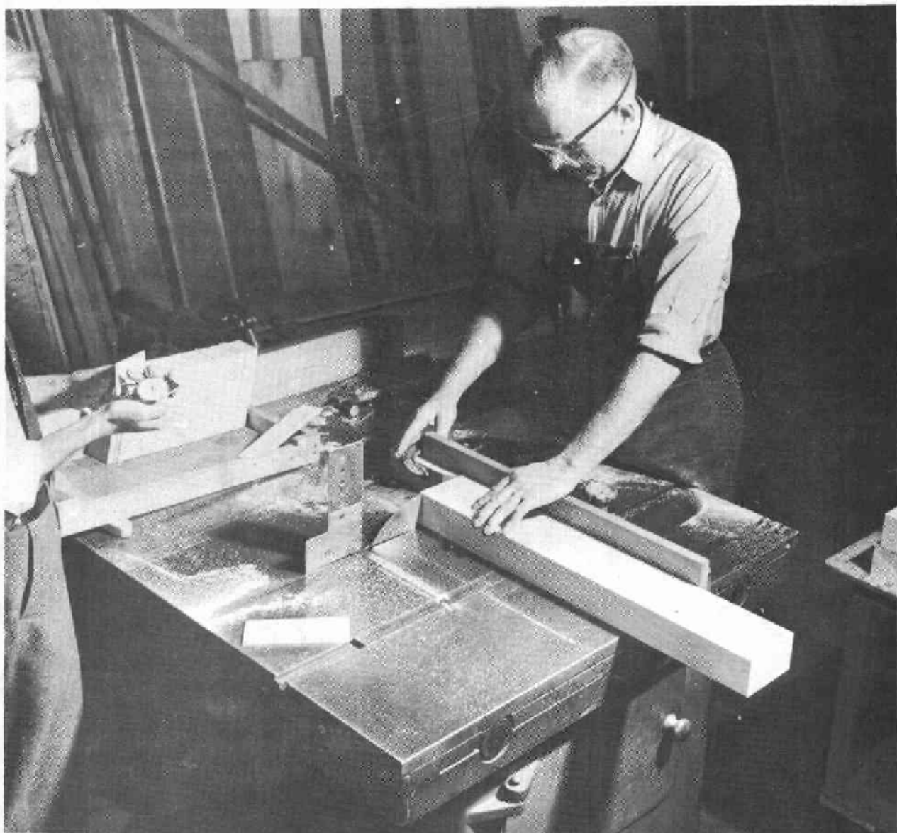
Figure 3.--Table saw set-up for cutting end-grain balsa core stock.
