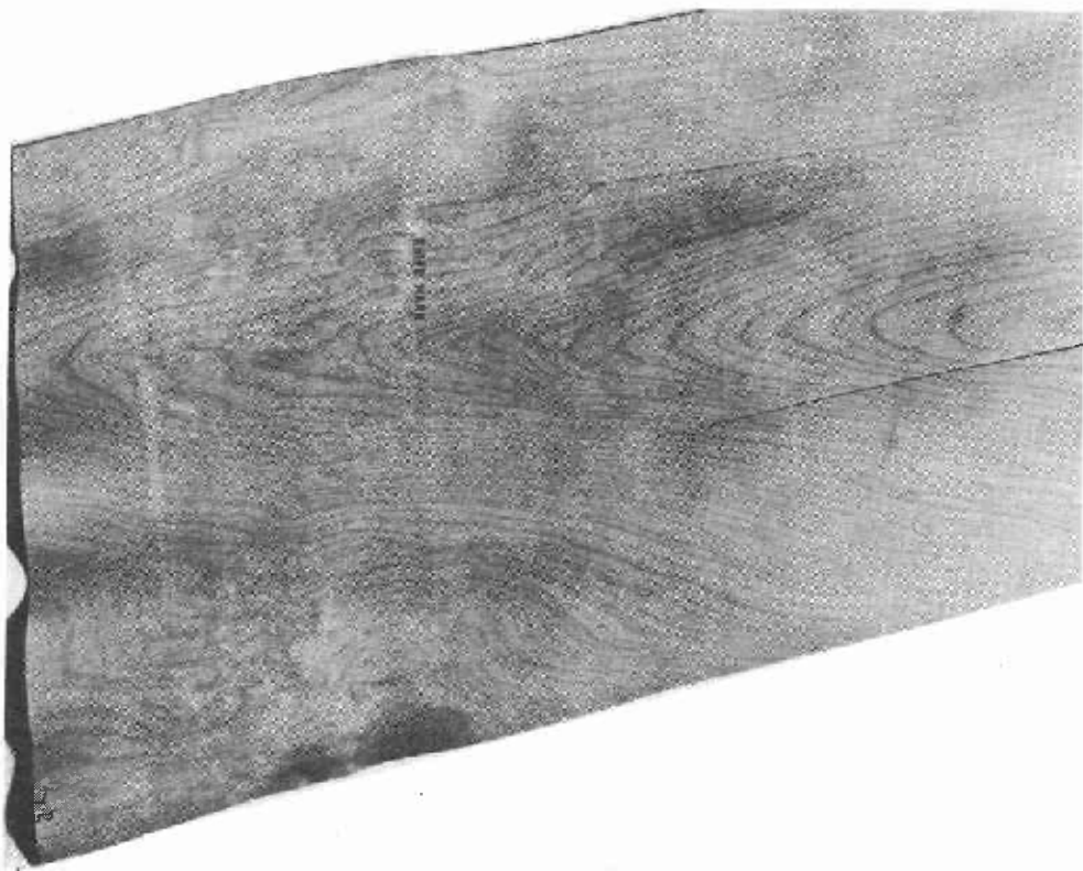
Figure 32.--Rotary-cut birch veneer showing broad annual ring pattern across the grain and knife marks at right angles to the edges; also spiral grain as indicated by split which is not parallel with alignment of apexes of annual rings due to diagonal grain.
