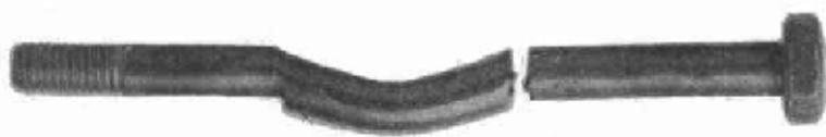
Figure 15.--Steel aircraft bolt sheared during bolt-bearing test of 1-inch cross-banded compreg under compressive loading. Ultimate load, 7,480 pounds; bolt diameter, 0.246 inch; bearing length, .949 inch.
