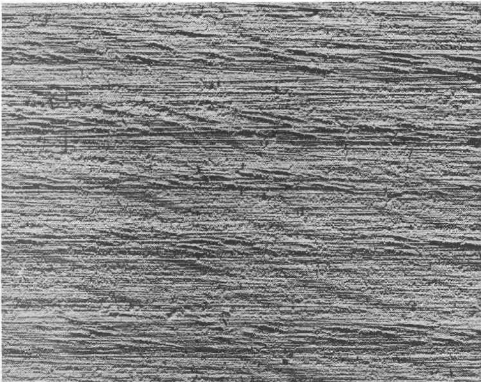
Figure 1.--Raised grain on surface of oak after sanding but not sponged. Magnified 4.1 times
