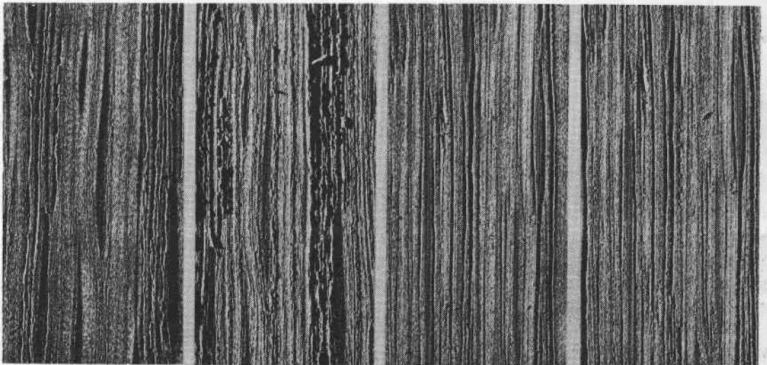
Figure 2.--Plain-sawed mahogany. Magnified 4.1 times ( a , Surface sanded but not sponged; b , same after sponging; c , surface hand planed but not sponged; d , same after sponging.)
