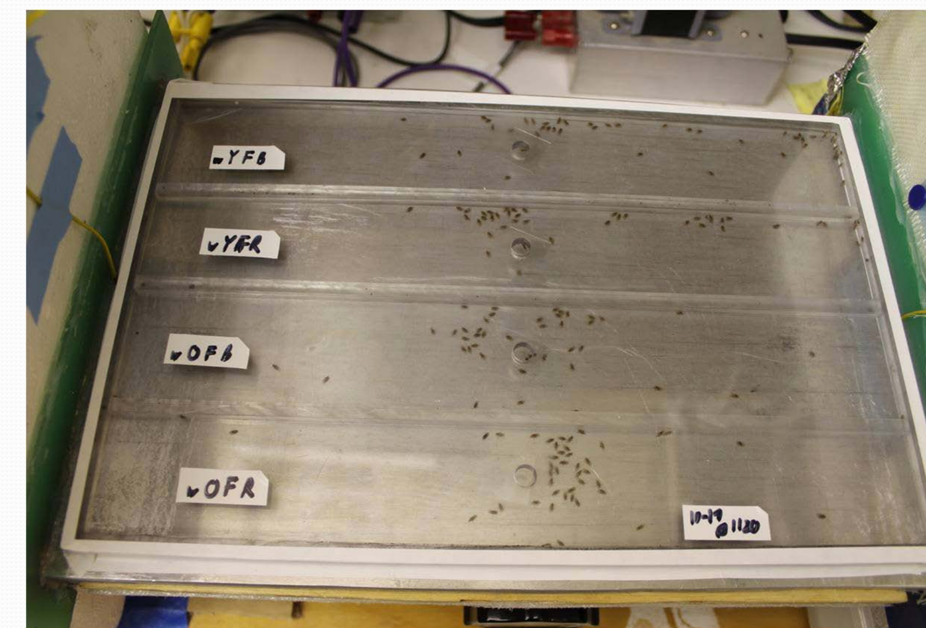
Figure 3. Schematic drawing of the temperature gradient apparatus used in the experiment. Flies were placed on the Aluminum plate under the plexiglass cover (C).
