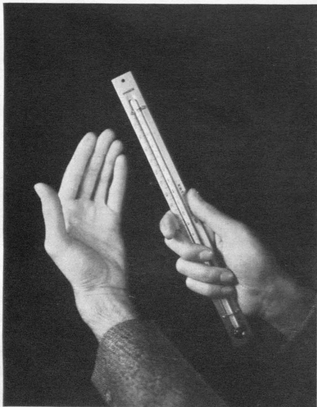
FIGURE 4.—Showing second process of reuniting alcohol column in minimum thermometer.
