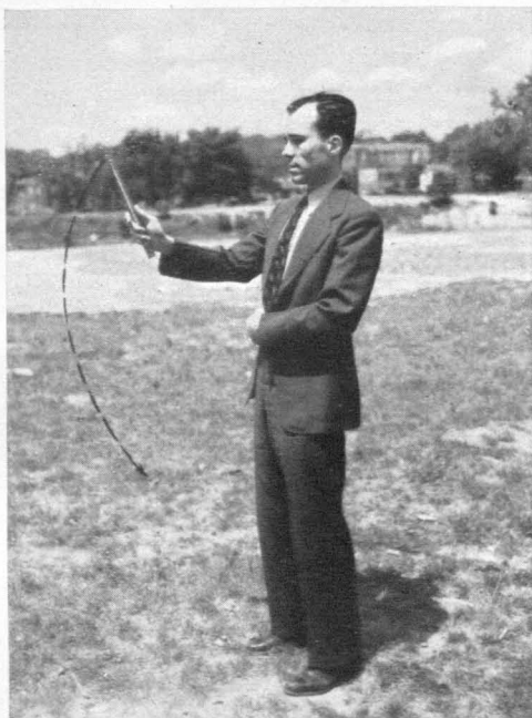
FIGURE 5.—Showing third process of reuniting alcohol column in minimum thermometer.
