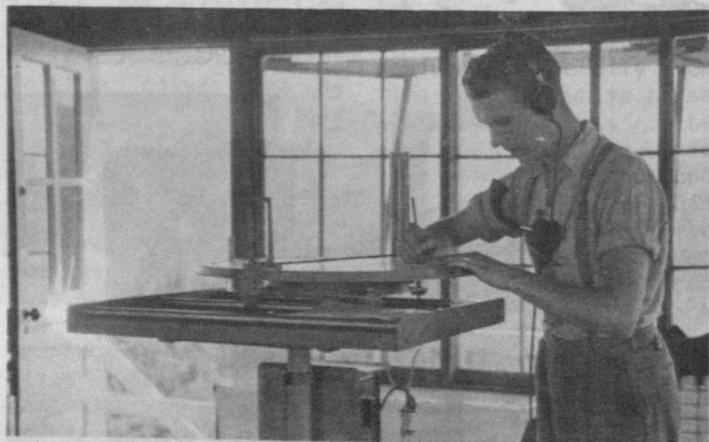
Lookout telephone headset frees the operator to complete forms while talking with other lookouts. Colt Mountain lookout, Coeur d'Alene National Forest, 1939.
