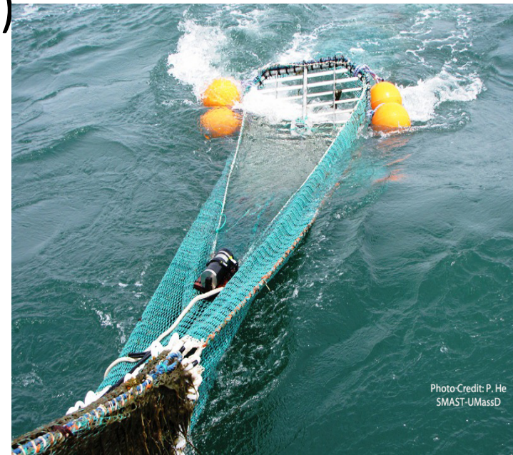
Grid to exclude fishfish from squid net
