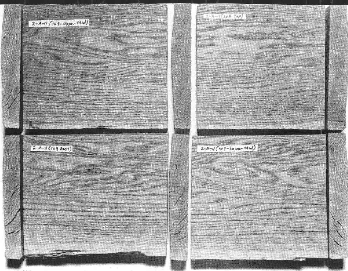
M 138 328 Figure 2. Ring failure in sections from a kiln-dried, FAS, 4/4-inch board of northern red oak that was bacterially infected when green. (M 138 328)
