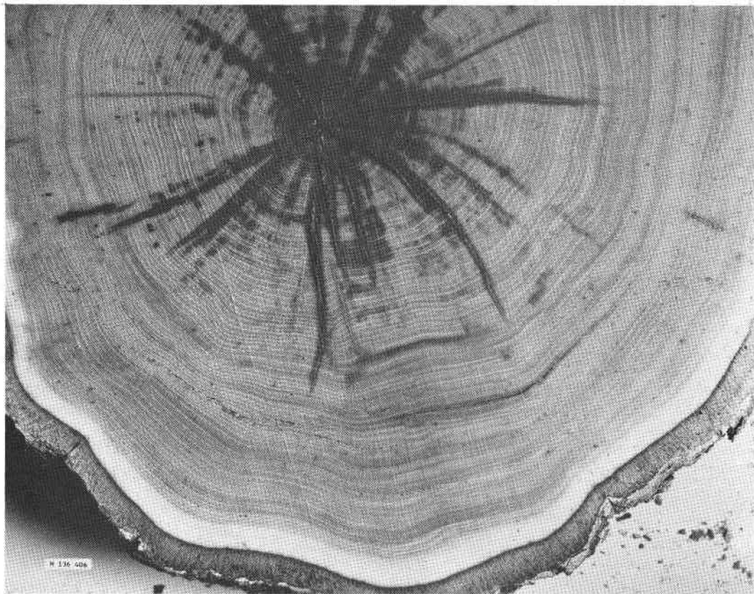
Figure 3. Stem section, 1 foot above ground, from a northern red oak tree showing a combination of both ring shake and spider heart (star shake). The sound, clear portions of the heartwood are infected with bacteria. (M 136 406)
