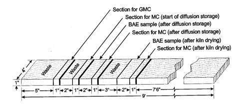
FIGURE 2. Sampling diagram for each board.
