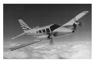
Fig. 7. Piper Seneca III light twin-engined aircraft instrumented and operated by the University of North Carolina at Chapel Hill.
