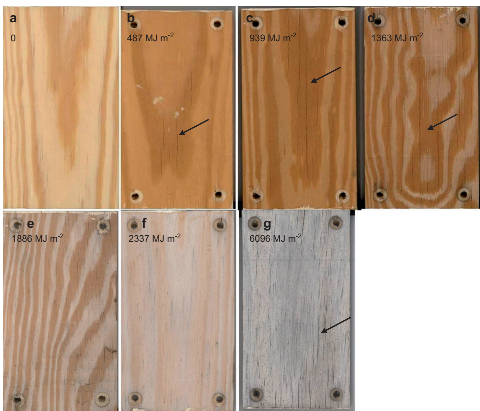
Figure 2 Photographs showing progressive check and discoloration development on untreated control loblolly pine sample (a) 0 and the samples (b–g) for the indicated irradiation doses.
