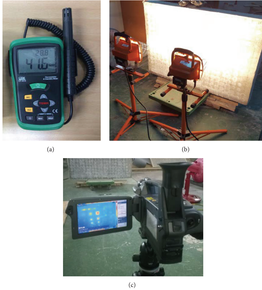
FIGURE 4: Equipment utilized in the experiment: (a) CEM DT-615, (b) Halogen lamps, and (c) IR thermal camera.
