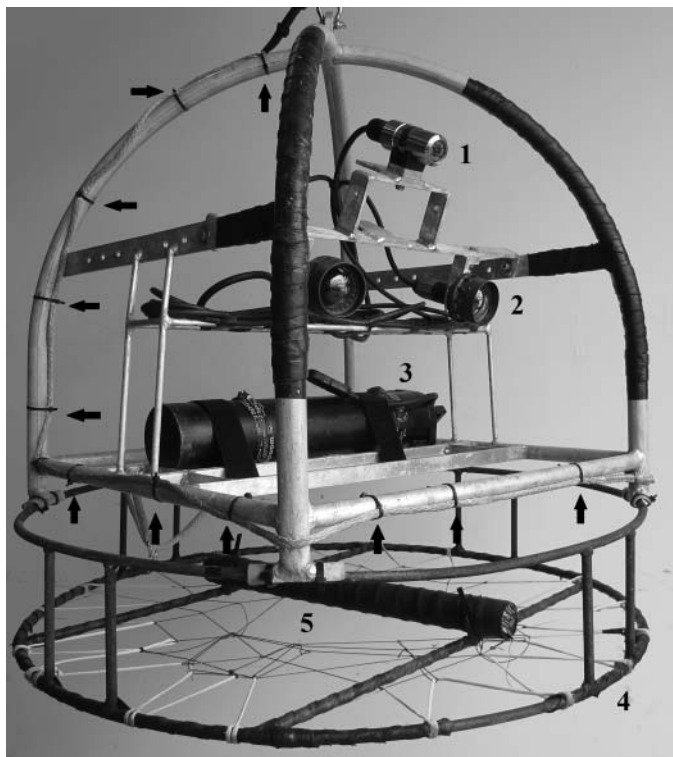
FIGURE 1. The video lander platform utilized at Three Arch Rocks reef. Displayed in the photo are the Deep Sea Power and Light (DSPL) Multi-Sea-Cam 2060 (1), dual DSPL LED Mini-Sealites (2), pressure tube containing batteries and Sony TRV-11 digital camcorder (3), sacrificial (breakaway) base (4), and steel-rod weight bar (5), with arrows showing the break-away connection points.
