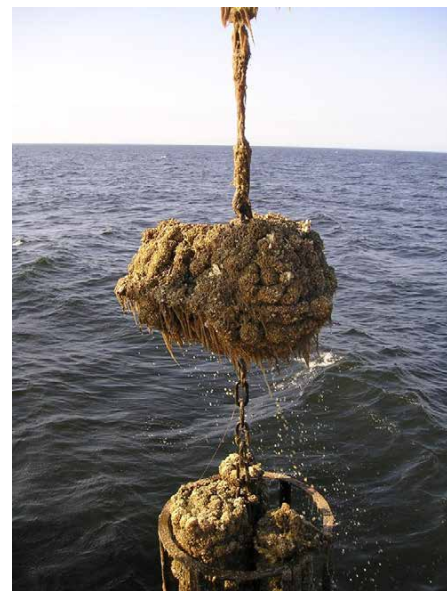
FIGURE 4. Recovery of mooring A3-03 (deployed from July 2, 2003, to August 31, 2004), showing heavily biofouled trifloat-flotation package (upper item) and NAS instrument package (bottom of photo). Photo credit: Rebecca Woodgate, University of Washington, taken from R/V Alpha Helix
