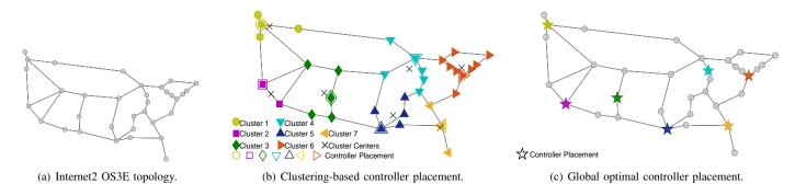
Fig. 3: Illustration of the controller placement decisions for k = 7 where the objective is to minimize the average switch-controller distance.
