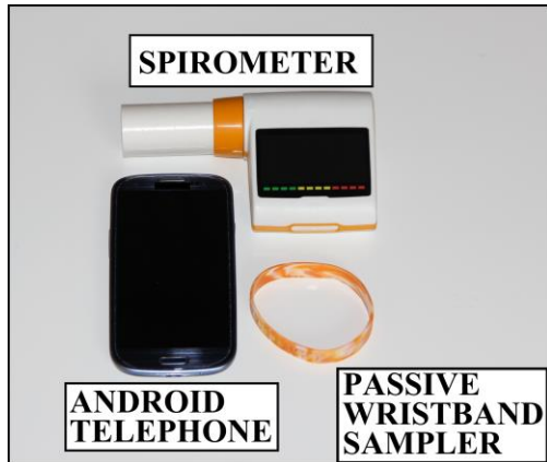
Figure 1. The ELF device is comprised of passive wristband sampler, an Android mobile phone with the ELF Tracker app and a portable spirometer.
