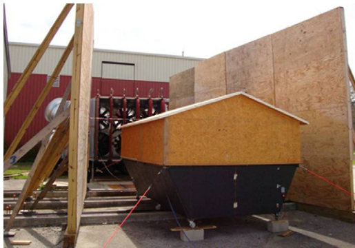
Fig. 4. 1/3-scale model building, wind generator prior to validation testing. (Model was tied down to minimize buffeting).
