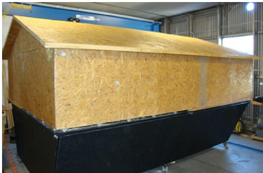
Fig. 2. 1/3-scale light-framed wood model building used in the study (wall pressure taps w1 and w2 are clearly seen on side wall).
