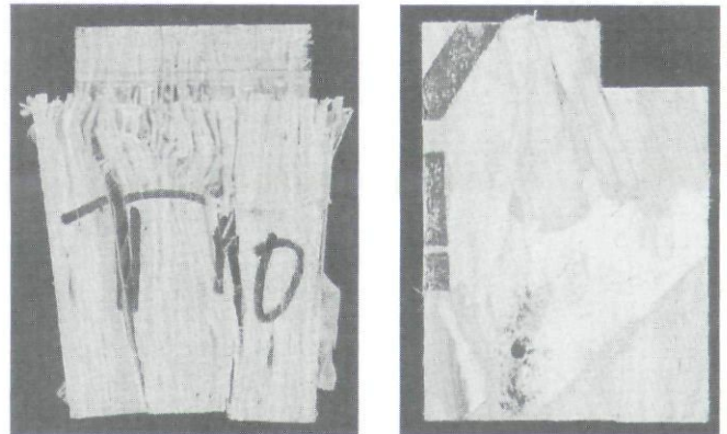
Figure 4. — Typical compression failure in joist-oriented LSL block.
