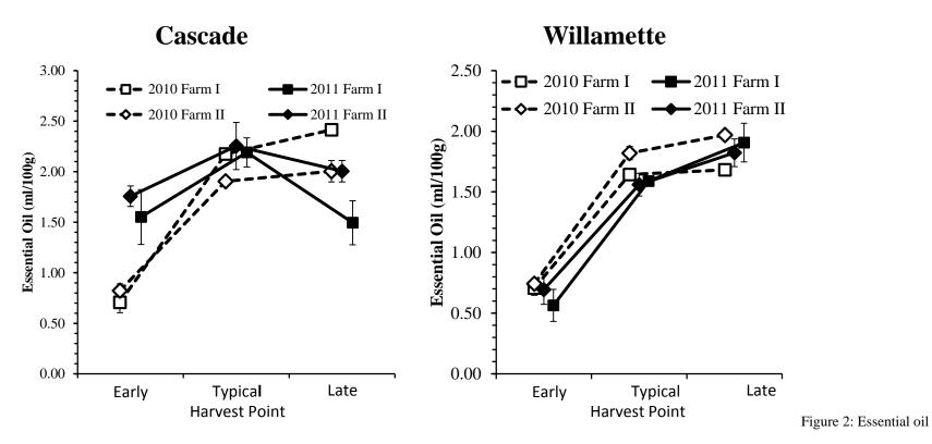
content of Willamette (left) and Cascade (right) hops at different harvest points by farm and year. Note, the more pronounced effect of year on Late harvested Cascade hops. Error bars represent standard deviation.
