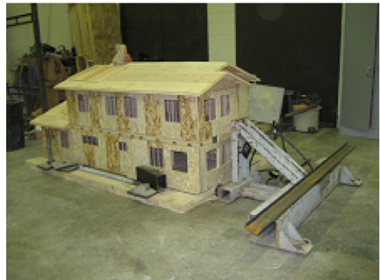
Fig. 8. Experimental setup at Colorado State University for determination of the load–deformation curve.
