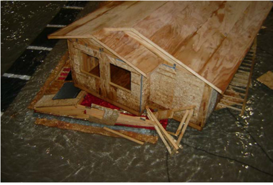
Fig. 9. Collapse of model in orientation B when subjected to the 60 cm wave. Note that there was 10 cm of standing water in and around the building. This water was not present during the majority of testing including the data used to determine the force equation constant in this study.
