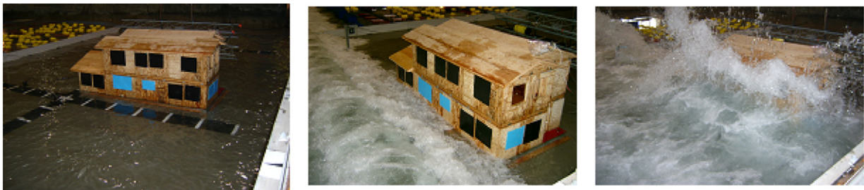
Fig. 4. Typical sequence photos of wave impact during TWB testing. The photos shown here are for a 50 cm wave.
