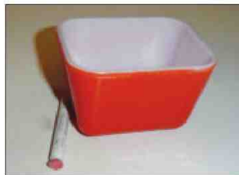
The paint on the outside of this small nesting casserole dish has lead in excess of 250 times current federal standards.
