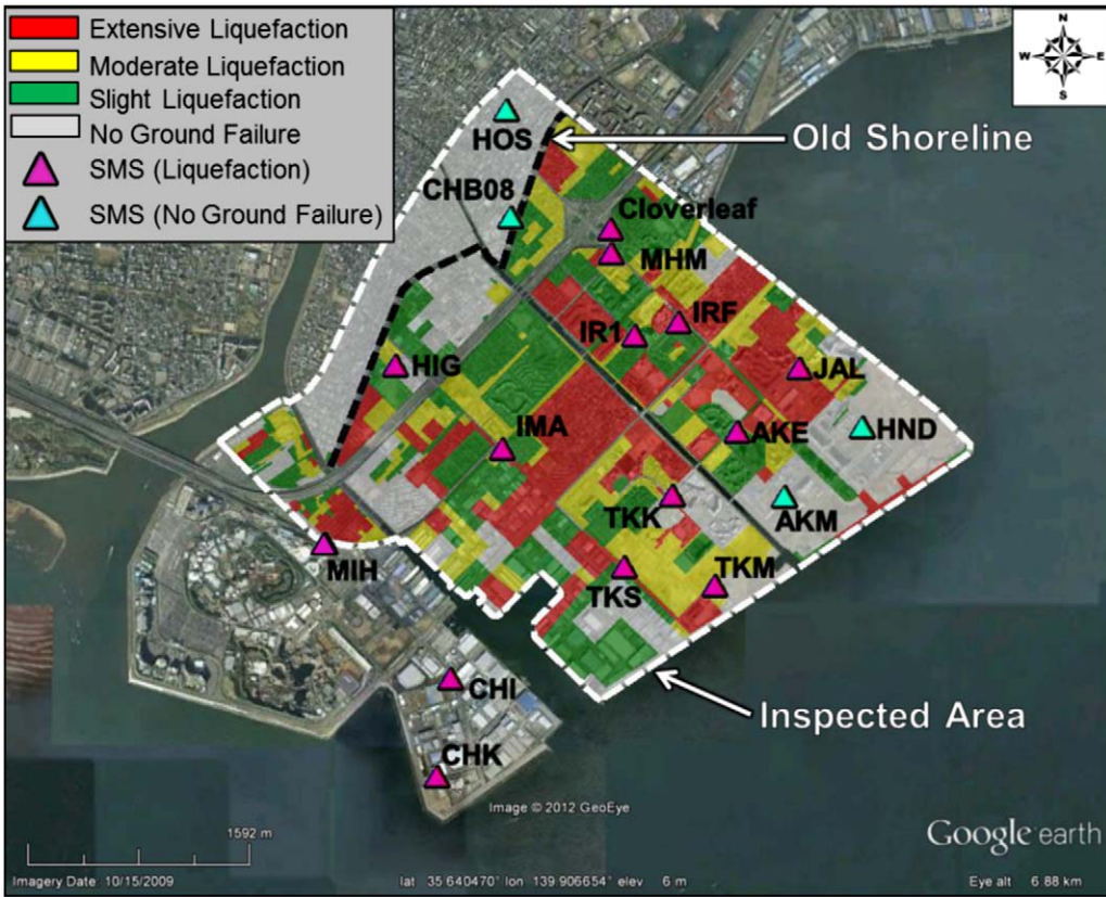
Figure 7. Liquefaction severity map of Urayasu City with the locations of strong ground motion stations (liquefaction severity after Tokimatsu and Katsumata 2012).
