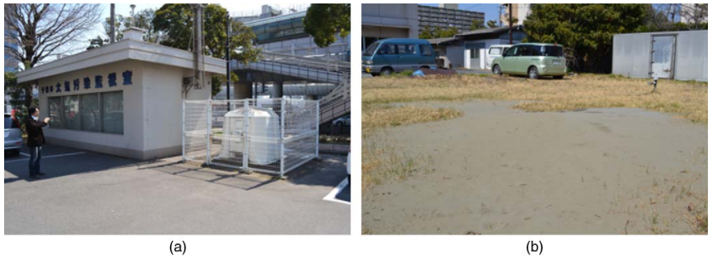
Figure 2. Two recording stations in Chiba: (a) station CH009 without ground failure, and (b) station CHB024 with extensive sand boils and moderate ground deformations.
