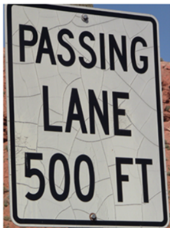
D. Cracking Damage
