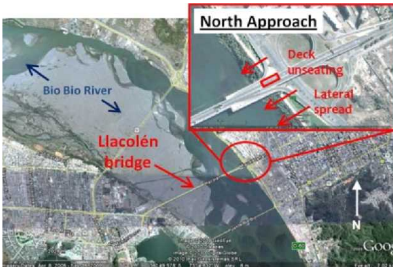
Figure 3. Plan view of the Bio-Bío River region, locating the damaged region of the Llacolén Bridge in Concepción ( S36.830108^\circ W73.067991^\circ ).
