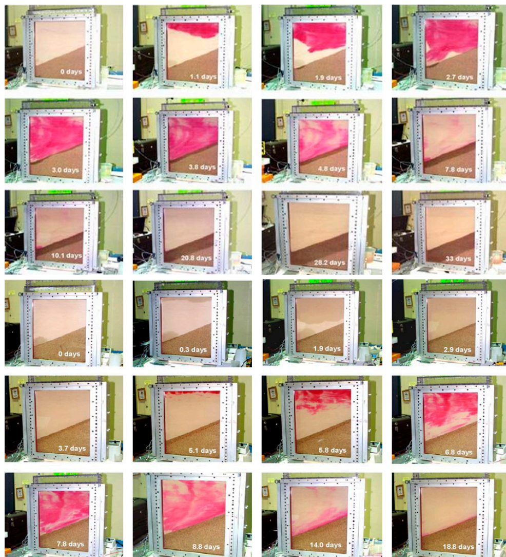
Fig. 6. Dye tracer transport time lapse for Exp. 1 (angular sand) (top) and Exp. 2 (round sand) (bottom).
