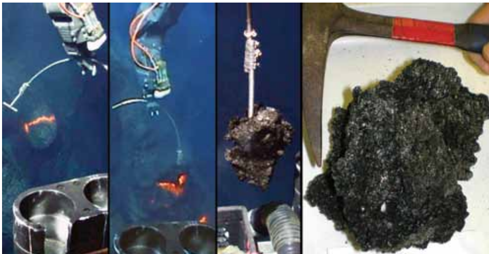
Figure 4. Images of the first molten lava sampled in the deep sea by the remotely operated vehicle Jason during the 2009 Northeast Lau event response cruise on R/V TG Thompson . The Jason team skillfully inserted a T-handled rod into a glowing portion of an advancing pillow lobe and pulled out a cantaloupe-sized piece of lava, subsequently shown to be a rare magma type known as boninite (Resing et al., 2011).
