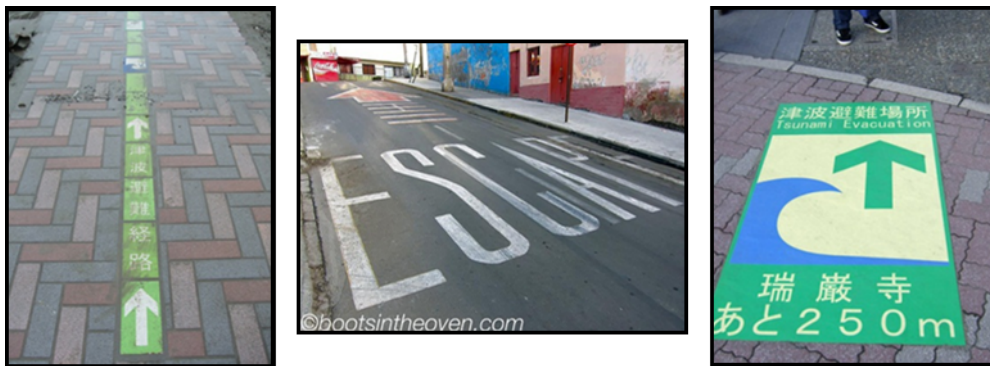
Figure 7: Tsunami Evacuation Route Pavement Markings
