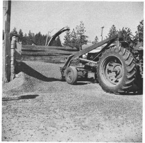
A tractor-mounted scoop used to load delivery vehicles.
