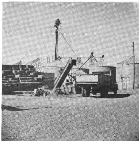
Self-unloading truck used to deliver shredded hay to feedlot. Machine in background is baled hay shredder.
