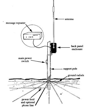
Components of a low power radio system. (Adapted with permission from Digital Recorders, Inc.)
