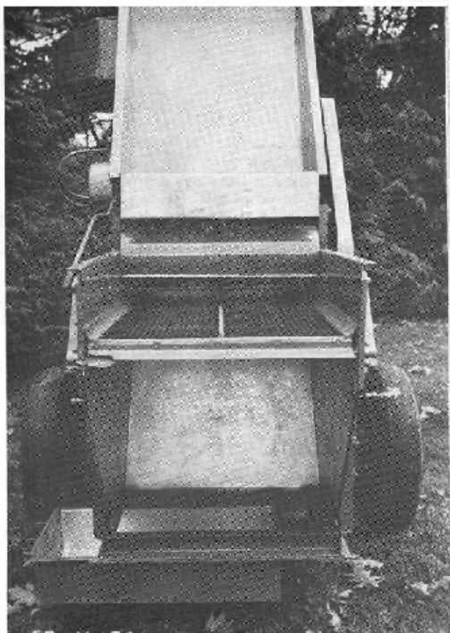
FIG. 3.—Experimental thresher with sieve hood raised, and a section of the seed chute removed exposing the sieve for inspection and cleaning.
