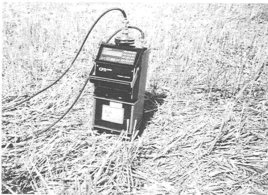
Figure 5. The neutron probe increased the speed and convenience of determining soil moisture
