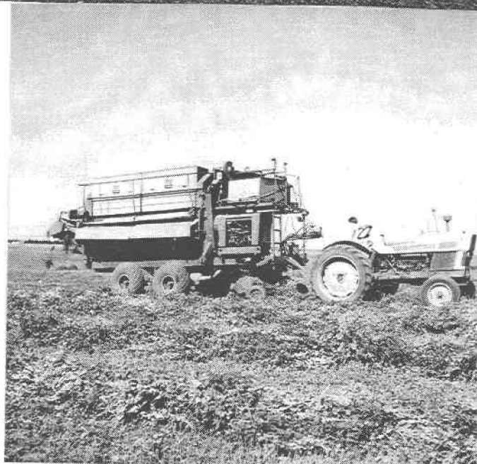
Figure 9. Pea vining changed from the stationary viner (top) to mobile field viners (bottom, an early model). Stationary pea viners became obsolete.
