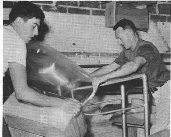
Figure 2. Worker at right is fitting liner on mandrel. Other member of 2-man team is stockpiling a lined box.
