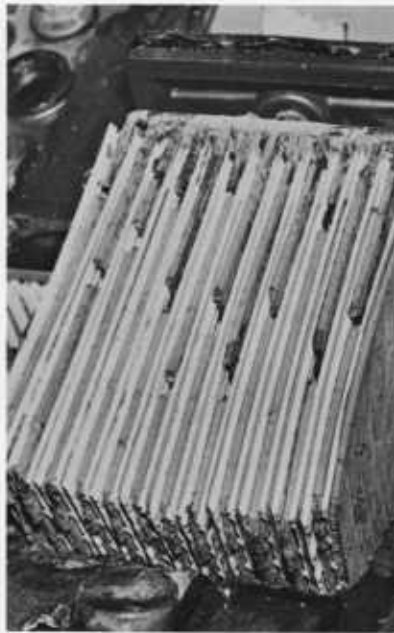
Lead sulfation occurs in any lead-acid battery. It can shorten battery life if a battery is allowed to sit discharged. The white at the bottom of these plates is lead sulfate. This cell sat discharged for a long time, with low electrolyte level. Lead sulfate built up prematurely, short-circuiting the plates and cutting the useful life of this battery.
