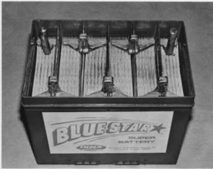
A heavy-gage lead strap connects adjacent cells across the cell wall. Cells are connected in series—from the positive side of one to the negative side of the second to the positive side of the third, and so on. The first and last connectors serve to install the battery in the circuit it powers.
