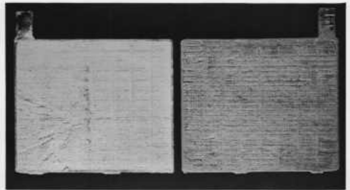
Positive plates (left) are filled with lead oxide, which is yellow. Negative plates (right) are filled with lead oxide and expander, and are gray. During the formation process, positive plates are converted to lead peroxide, which is brown. Negative plates are converted to sponge lead.
