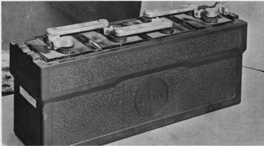
Regardless of the type of case used, each cell is sealed by the cover plate. Industrial batteries commonly locate the heavy-gage connectors between cells on the top. Smaller batteries usually have the connectors inside, beneath the cover plate.
