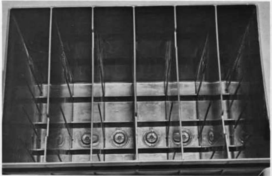
Raised ribs run across the cells along the bottom of the battery case. They support the weight of the plates and provide space at the bottom of the case. This space allows byproducts, that form as the battery works, to fall clear of the plates and not short-circuit the cell.
