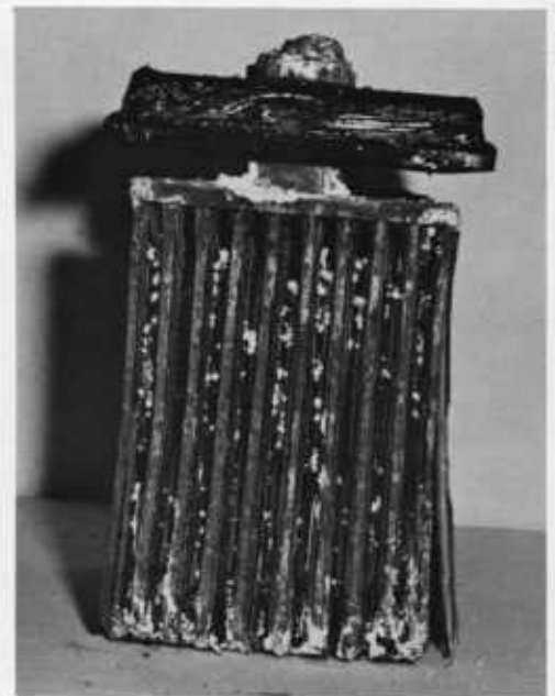
Sulfation can do mechanical as well as chemical damage. When batteries are allowed to sit discharged for long periods, sulfation attacks the grid structure of the plates. The positive plates of this cell were broken by sulfation expansion. The damage to this battery occurred as it sat on a boat in the discharged state for 1½ years.
