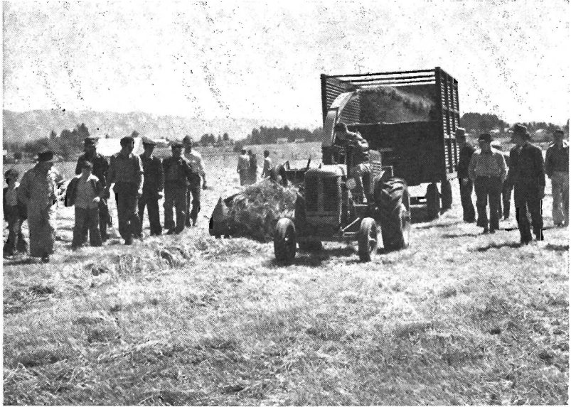
Figure 5. Demonstrating the use of a field chopper on a cooperator's farm. This outfit eliminates almost all hand labor and allows an operator to do his own work without hiring extra help. In some cases groups of neighboring farmers have purchased field choppers and shared the cost.
