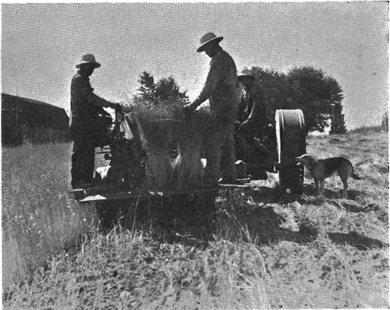
Figure 3. A MECHANICAL FLAX PULLER IN OPERATION. The puller crew usually consists of three men, including the driver of the tractor.
