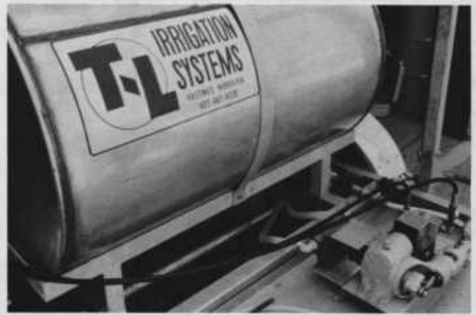
Figure 6.—Piston-type chemical injection pump and tank
