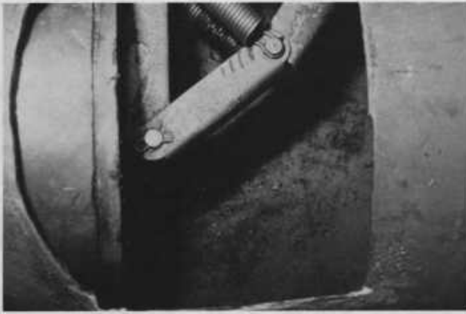
Figure 3.—Cutaway of check valve
