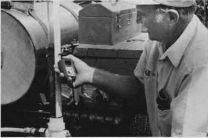
Figure 11.—Checking injection rate with a clear calibration tube
