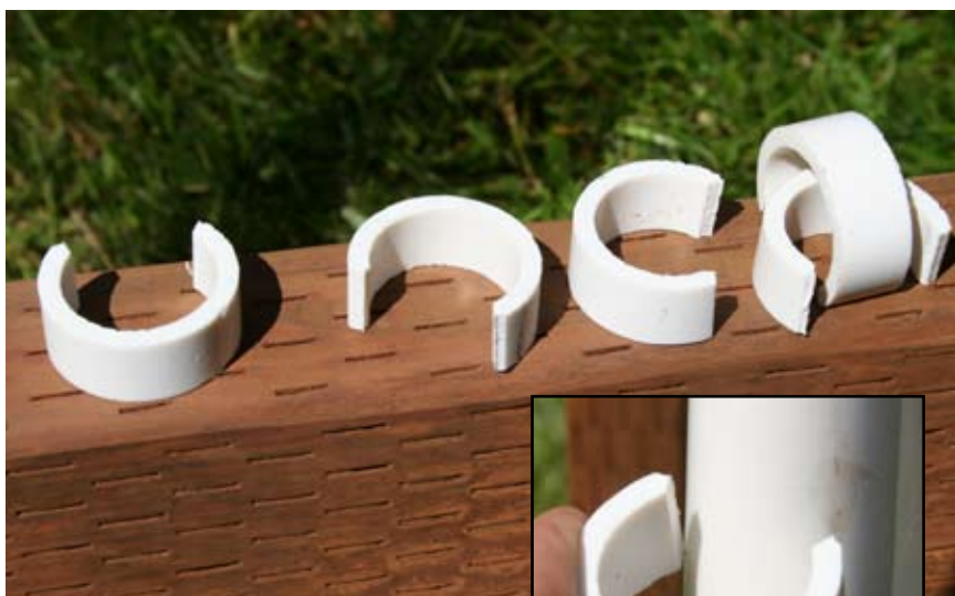
Figure 7. PVC clips for attaching polyethylene plastic sheeting to the ends of the cloche.
