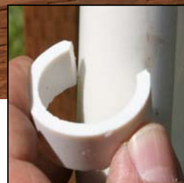
Figure 7 insert. Attach PVC clips to hoop.
