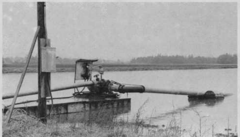
Do not wait until the storage pond is full to begin to sprinkle on cropland. Pump down liquid hold facilities when the weather and crops permit.
