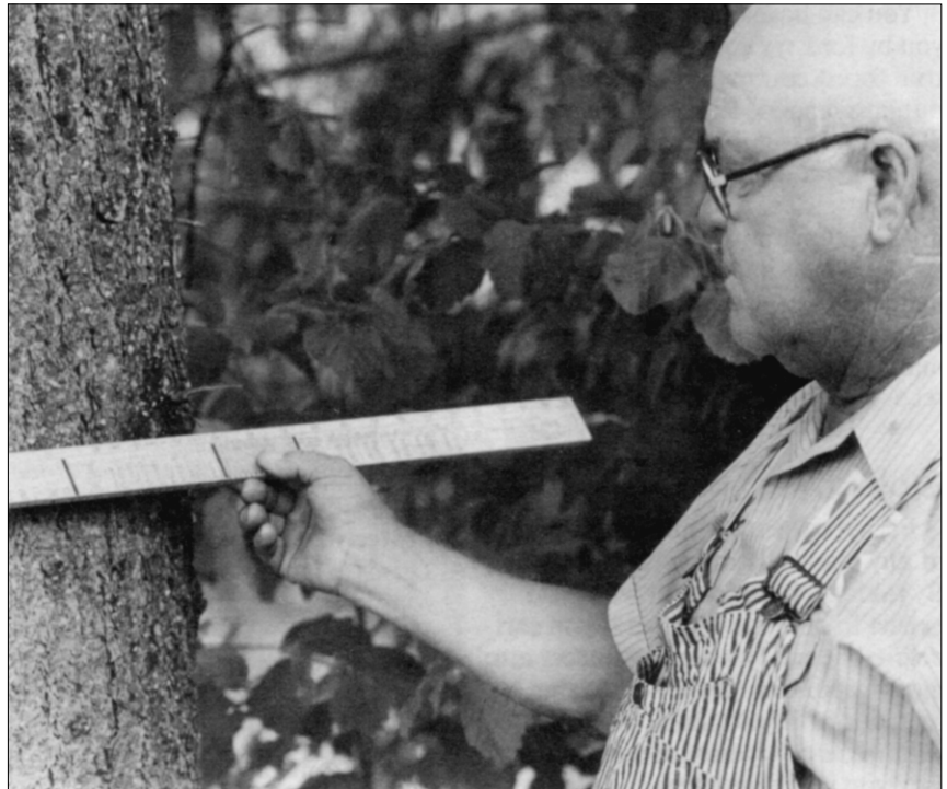
Figure 6.—The woodland stick is a handy tool to use in forest inventory.
