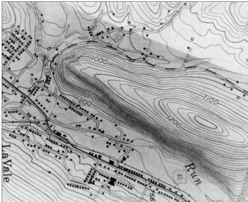
Figure 4.—Topographic maps show contour lines, constructed improvements, and other features.
