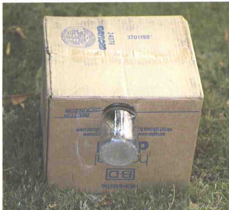
Figure 8.—A simple but effective emergence trap for monitoring needle midge emergence.
