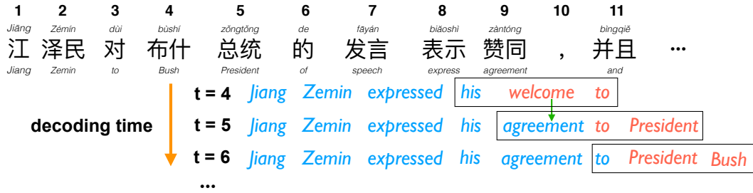
Figure 3.9: Decoder generates the 4 th word “his” and two extra words “welcome to” at the 4 th decoding step and the 9 th source word “zàntóng” (agreement) on source side is not available to the model yet. When the model receives the 9 th source word at 5 th step, the decoder immediately corrects the previous mistake with “agreement” and makes two more additional decoding. The decoder not only is capable to fix the previous mistake, but also has the enough information to perform more correct generations. Our framework benefits from opportunistic decoding with reduced latency here. Note though the word “to” is generated in step 4, it only becomes irreversible at step 6.
